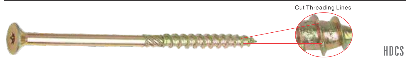
ST-203 HEAVY DUTY CHIPBOARD SCREW Countersunk Head Torx recess, 6 Ribs under Head, Cut Threading Lines
