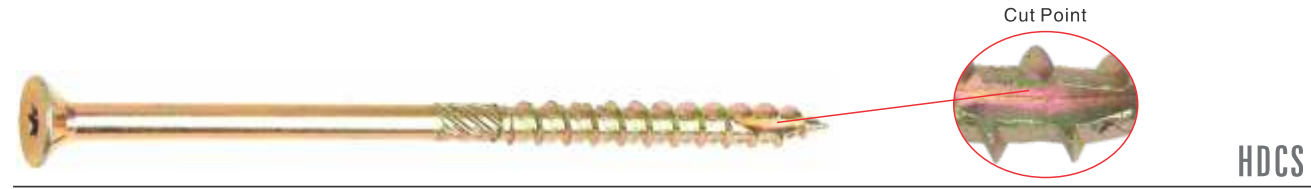
ST-202 HEAVY DUTY CHIPBOARD SCREW Countersunk Head Torx recess, 6 Ribs under Head,Cut Point
