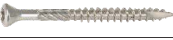
ST-1903 CHIPBOARD SCREW Countersunk Oval Head, Stainless Steel Torx Recess, 6 Ribs Under Head, Cut Point Cut Threading Line
