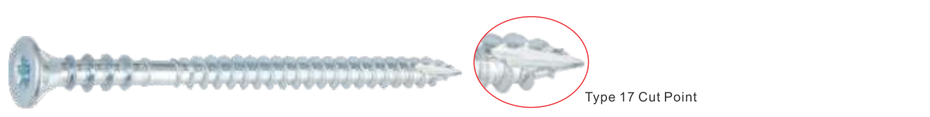
ST-18002 CHIPBOARD SCREW Countersunk Head Torx 6 Ribs under Head,Cut Point
