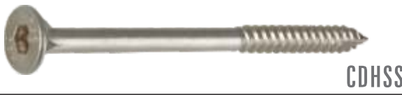
ST-1902 CHIPBOARD SCREW Countersunk Head, Stainless Steel Hex Recess, 4 Ribs Under Head, Cut Point
