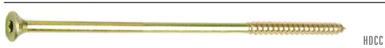
ST-205 HEAVY DUTY CHIPBOARD SCREW Countersunk Head Torx recess, 6 Ribs under Head,Normal Sharp point
